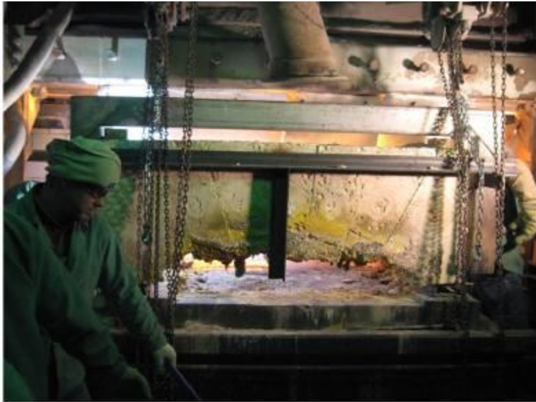
Existing mantle block being removed
